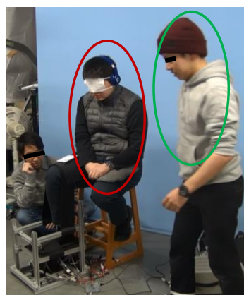
Fig. 9 Photo of the experiment for motion recognition. The person of the right side is an experimenter who performed motions. The person of the center is a subject who wore a blindfold, a headphone, and the developed plantar haptic display on the right foot.
