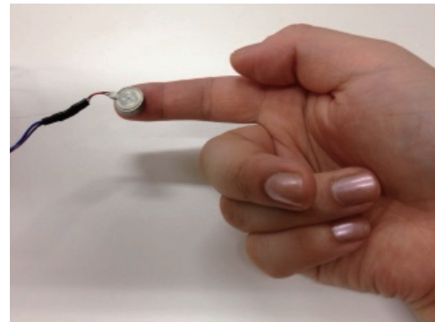
Figure 5. The part of the vibration system to produce the illusory force and finger movement for the index finger.
